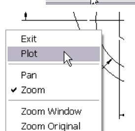
\*\*During PREVIEW right-click and select either "Exit" (to make corrections to the drawing) or "Plot" to send the drawing along to the plotter.
